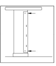
6. Use 1002499 Torx Screws - 7/16" to secure Alcove Joggle Bracket to 1/2" Thick Panel.
